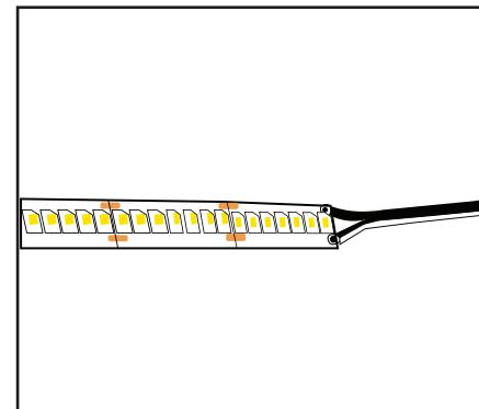
6. Once each point has been glued, push the endcap onto the end of the profile.
