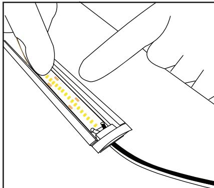
9. Place the LED Strip into the center spline of the profile, aligning the pre-soldered tail with the routed out wire exit.
