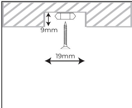
3. Mark and pre-drill screw holes prior to inserting mounting screws through Mounting Clips.
