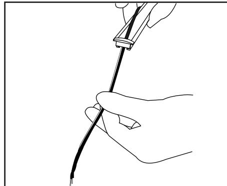
4. Thread the LED Strip wire through the routed out section of the profile prior to attaching endcap.
