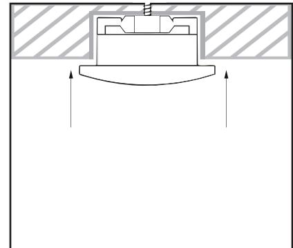
11. Pivot the front down and push firmly to engage the front of the bracket and snap-fit.
