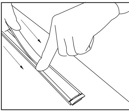
12. Push diffuser into the profile at one end then gently press along the rest of the length to secure into profile.
