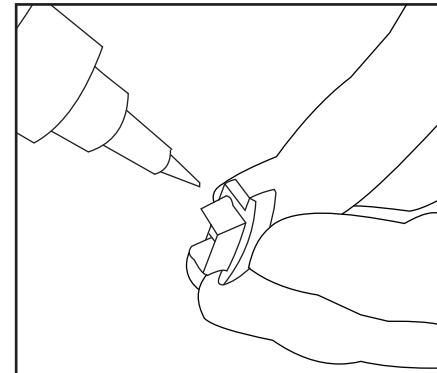
5. Using the Loctite 460 Instant adhesive or similar, dab some glue in each corner making contact with the profile.
