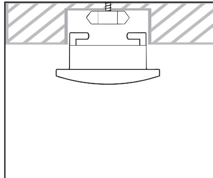
10. The assembled luminaire must now be attached to the mounting clip.
