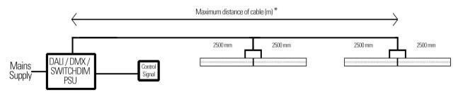
\* Power supply unit (PSU) output cable size 0.5mm<sup>2</sup> 0.75mm<sup>2</sup> 14m (mm<sup>2</sup>) / Max distance (m) recommendations: 1.0mm<sup>2</sup> 19m 1.5mm<sup>2</sup> 28m
