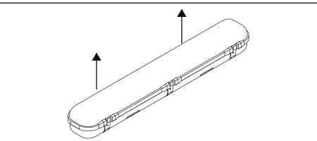
1. Remove the top cover/diffuser by releasing the toggle clips.
