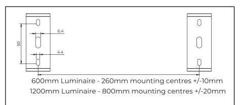
3. Fix the mounting clips with appropriate fasteners to the mounting surface.
