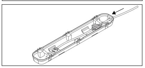
4. Insert mains cable through the M16 cable gland and tighten, to ensure ingress protection is maintained.
