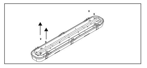
2. Partially loosen the hex head screws, which will allow removal of the gear tray. Unplug the yellow connector/s and put the gear tray carefully to one side.
