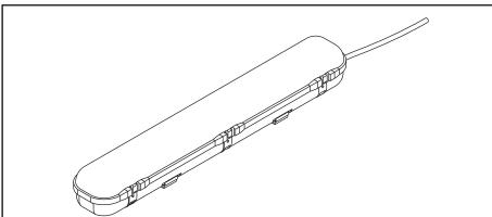
5. Re-attach the top cover/diffuser with the toggle clips.
