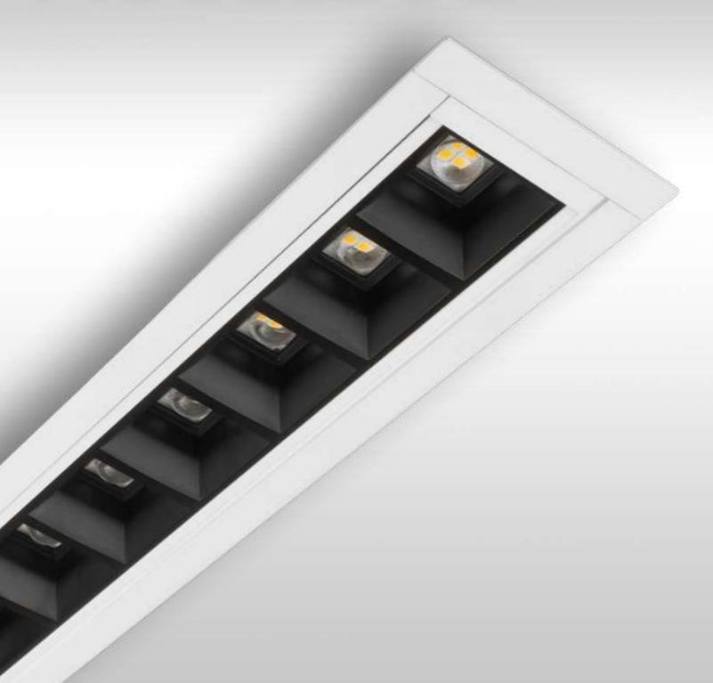
The Versatile VL9050 Louvered luminaire features an office-compliant UGR rating of <19, combining style with functionality. It offers four CCT options, including Tunable White, delivering up to 3,475 lumens per meter. With Non-Dim, DALI, and Casambi control options as standard, and a variety of louver colours available.
