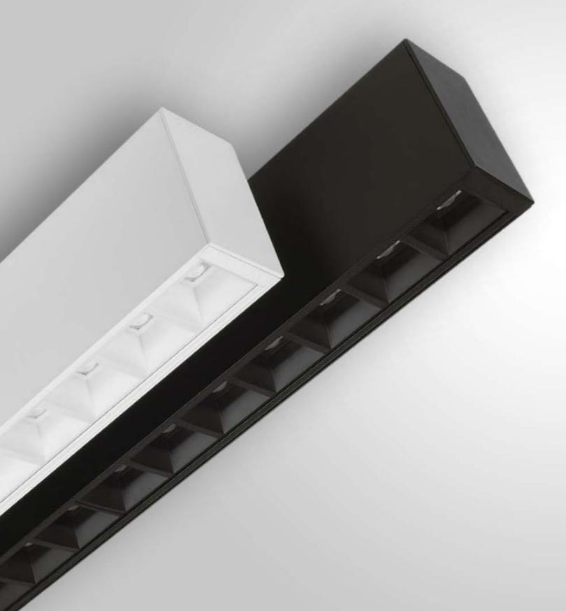
The Versatile VL9050 Louvered luminaire features an office-compliant UGR rating of <19, combining style with functionality. It offers four CCT options, including Tunable White, delivering up to 3,475 lumens per meter. With Non-Dim, DALI, and Casambi control options as standard, and a variety of louver colours available.
